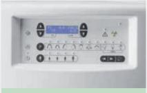
**Simple Operation**Simply select program (8 Pan or 3 Ceph) and patient size (4 options). All exposure settings will be set automatically. Presets can also be adjusted manually.
